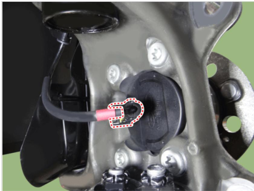
3. Loosen the wheel speed sensor bracket bolt (A), and then disconnect the wheel speed sensor connector (B).
